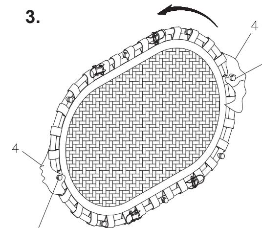
**B.** Second step, install the Safety Pad(4) on the opposite end being sure the hole fits over the threaded connector.
