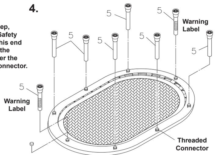
Remove all of the eight Plastic Caps from the threaded connectors before installing the LEGS(5).
