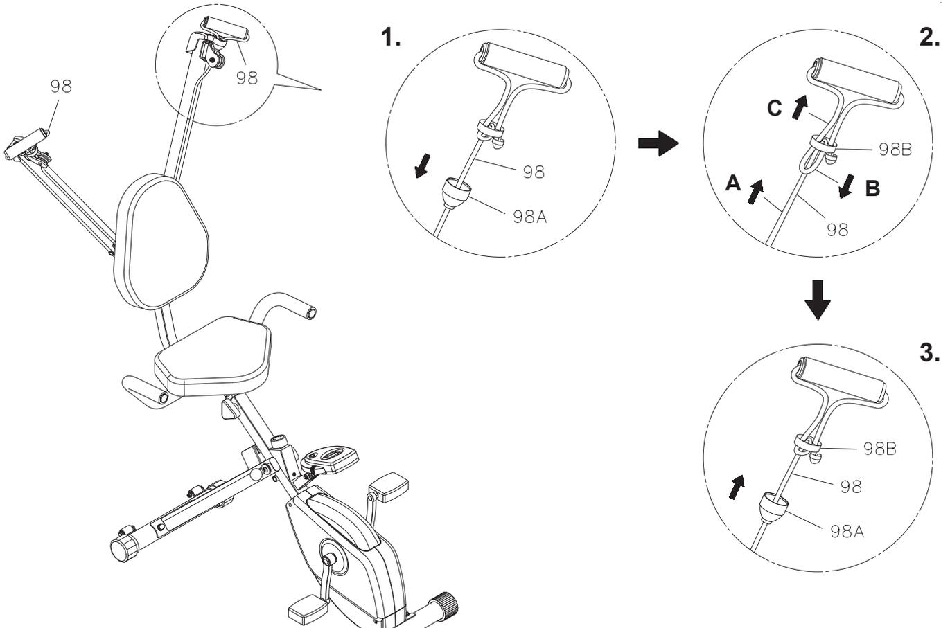
1. Pull the **TENSION CORD(98)** away from the pulley slightly. Slide down the **COVER(98A)** as shown in **View 1**.
